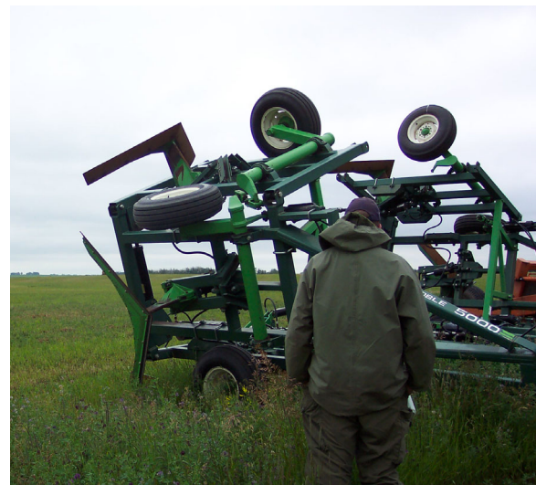
Nobel blade cultivator breaks the connection between root and shoot, but leaves stubble standing. Photo by Brenda Frick
