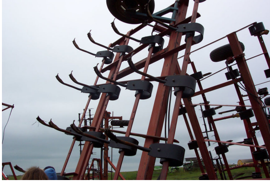
Quack grass cultivator (right) pulls quack grass rhizomes from the soil. Photo by Brenda Frick
